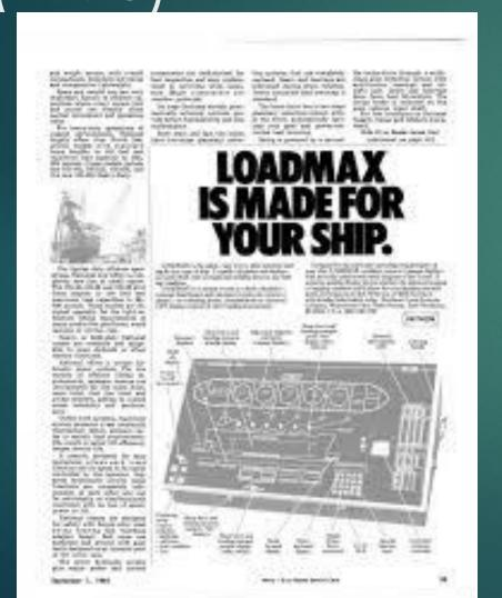
These instruments were the first to be microprocessor based using the Intel 8080 CPU, LED numeric displays, silk screened mimic, the program was burned into EPROM chips.
