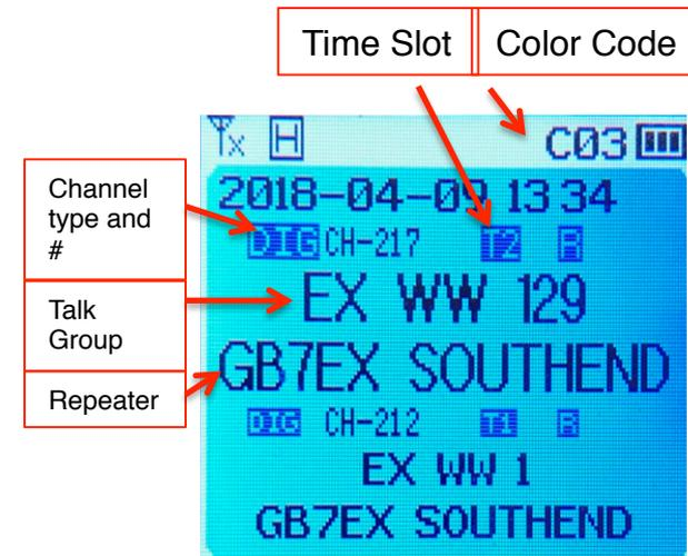
*Typical DMR radio screen showing a primary and secondary channel. Both are on the same repeater, but on different talk groups.*
