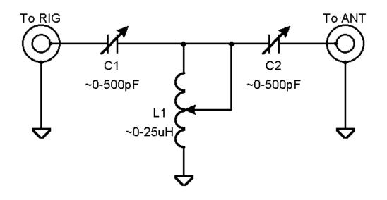
Fundamentally it is an variable impedance matching circuit.
