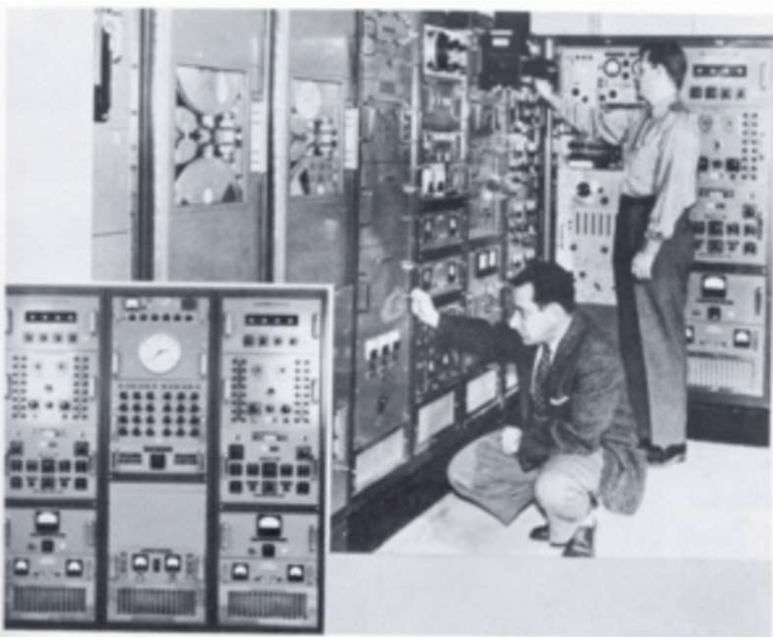
FIGURE 45.—The TIROS I command and data-acquisition station at Fort Monmouth, N.J., and (insert) the satellite programming racks, which are cut off at the right of the main picture.
